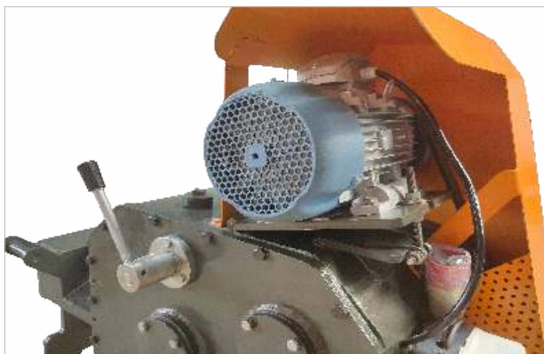
S1 duty motor for continuous operation
