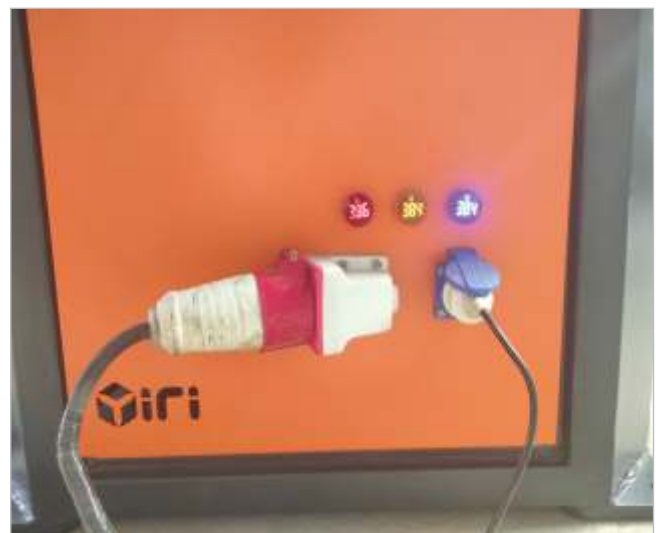
Special Voltage indicator provided to check the incoming power. This helps prevent motor and electrical damage due to power fluctuation
