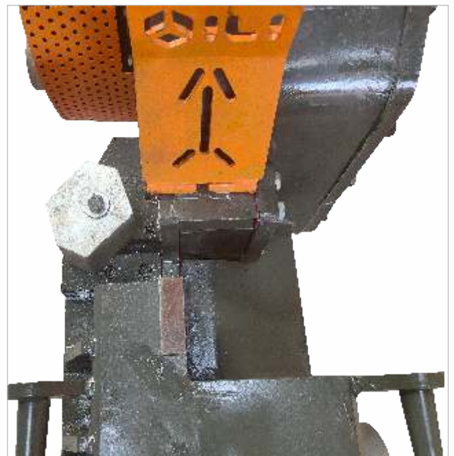
Special rubber seal provided to minimize oil leakage from cutting area
