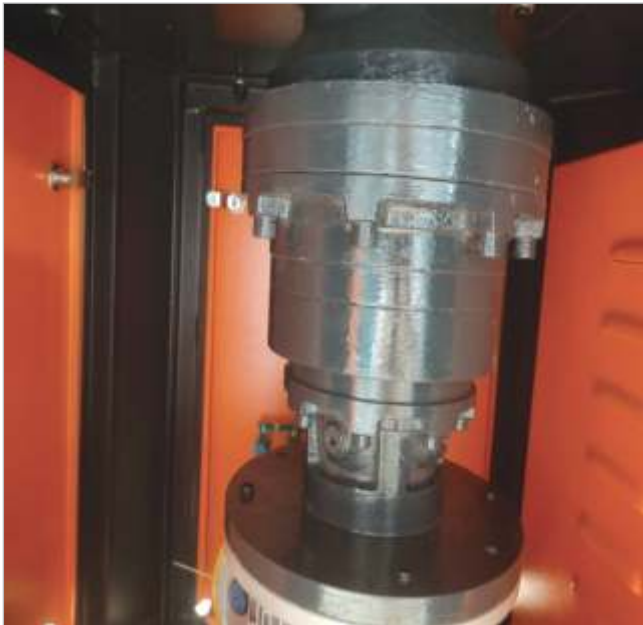
Planetary gear box with high torque for smooth operation.
